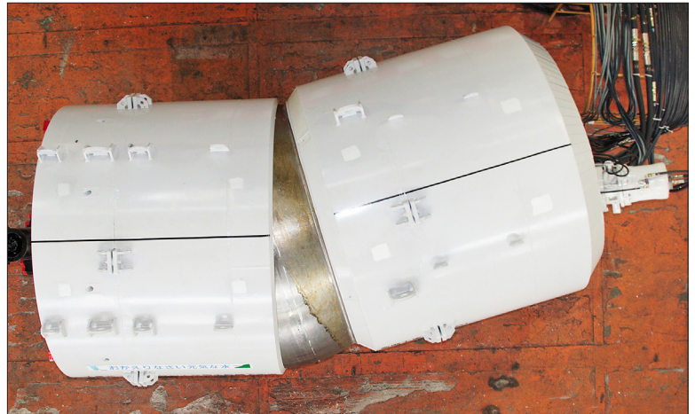
Figure 5. A fully-articulated tight radius curve TBM.
