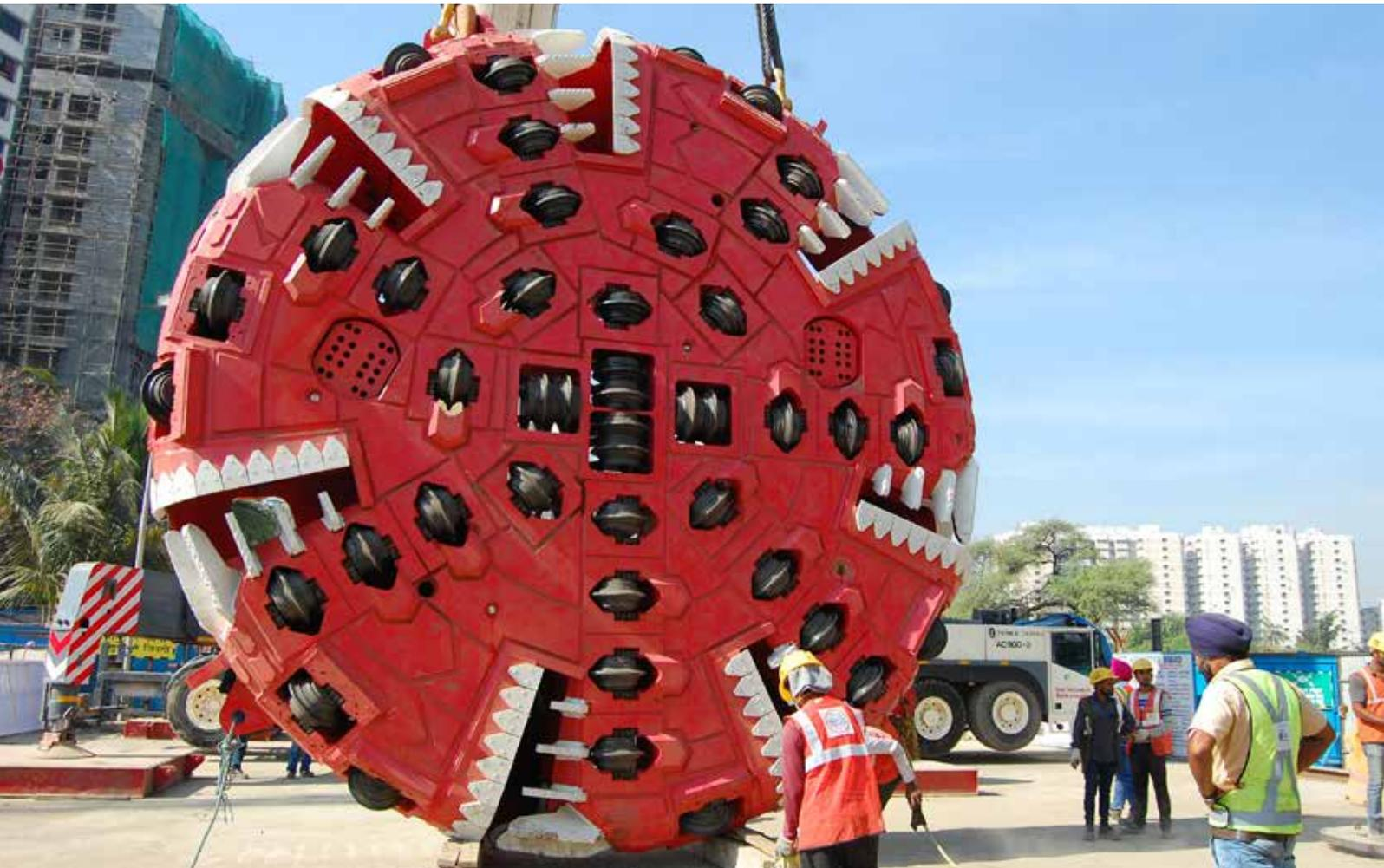
**I**n early August, TERRATEC celebrated the assembly of its fifth new 6.68m diameter dual-mode hard rock TBM to go to work on Mumbai Metro's Line 3 project, in India, at the CSIA International Airport shaft on contract UGC-06. The first four of these machines are fully up and running on two other contracts (UGC-02 and UGC-05) and achieving production rates of up to 91m per week.
